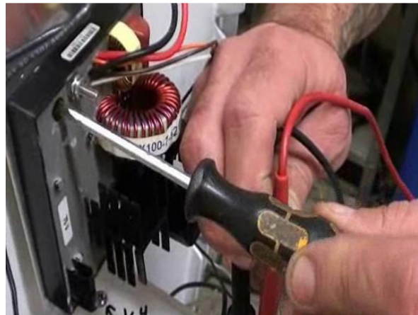
Above: Using a flathead screw driver to adjust the power 9.5V DC at the lowest step.
