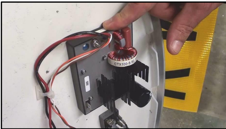
Left: E410 (50V) or E610 (75V) Controller Located on the top right of the end panel.
