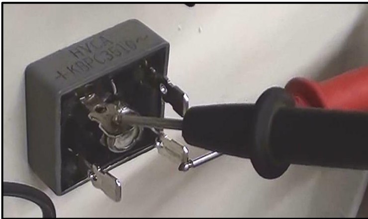
Above & Right: Testing the Bridge rectifier (multimeter on diode setting)
