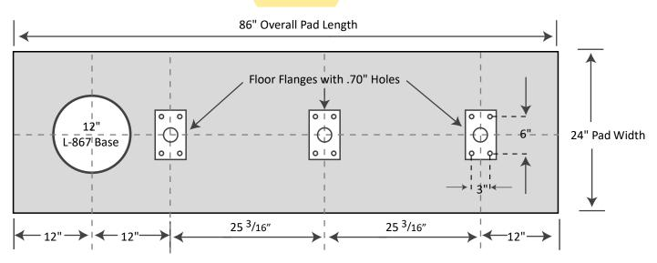
Use 5/8" diameter anchor bolts for mounting to pad
