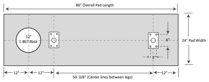
Use 5/8" diameter anchor bolts for mounting to pad When setting bolts, allow for approximately 3/4" flange thickness.
