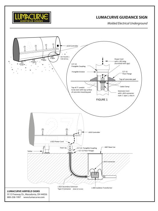
with a DC voltmeter after installation. Lamp voltage is read across the white and brown leads at the sign terminal strip on the light bar (P/N #CLT 8A). If voltage varies from recommended settings (9.5V at lowest CCR step for all size signs), all signs on that circuit should be checked and adjusted. To adjust, turn the small screw in the upper left corner of the printed circuit board (E610) controller mounted on the inside of the end panel (P/N #CLT-4).
