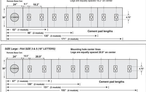
Above references recommended cement pad dimensions and mounting bolt locations for Lumacurve signs \*Recommended concrete thickness : 6"-8" \*Recommended anchor bolts: 3/8" x 5" with LOCK washers
