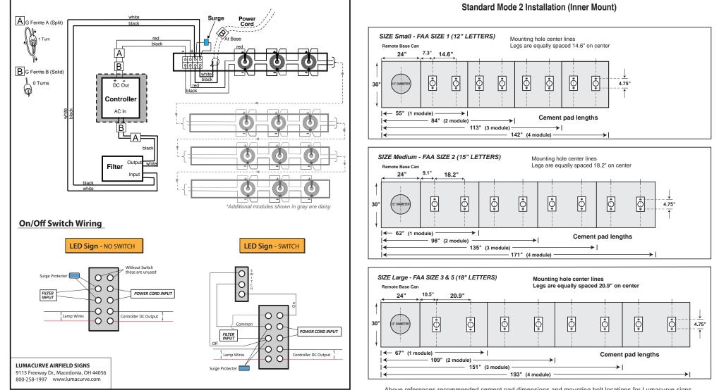
Above references recommended cement pad dimensions and mounting bolt locations for Lumacurve signs \*Recommended concrete thickness : 6"-8" \*Recommended anchor bolts: 3/8" x 5" with LOCK washers
