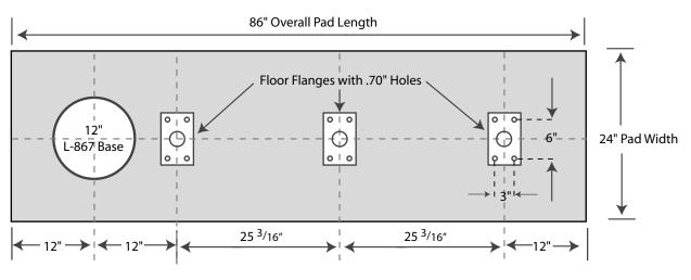
Use 5/8" diameter anchor bolts for mounting to pad When setting bolts, allow for approximately 3/4" flange thickness.
