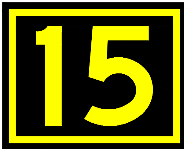
(b) Runway Location Sign
