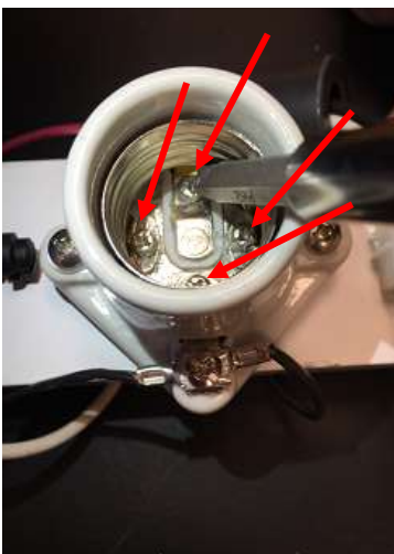
Figure 1, tightening the 4 socket screws
